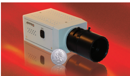
▲ DMVA2IPNC-MT5 IP Camera Reference Design available from Appro Photoelectron Inc.
