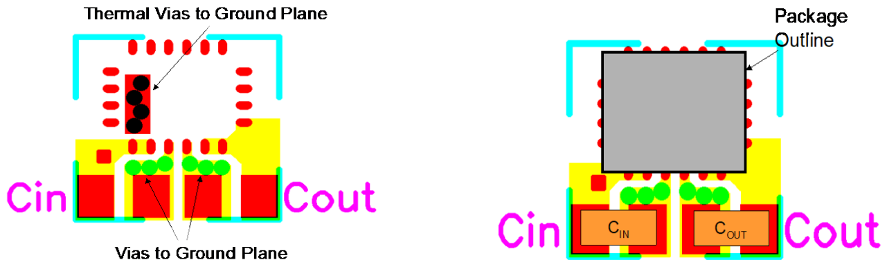
Figure 8. Example layout showing PCB top layer, as well as demonstrating use of vias from input, output filter capacitor local grounds, and thermal pad, to PCB system ground
