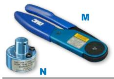
For crimping size #16 shield sleeves. These mil spec approved tools feature a ratchet mechanism to prevent damage from over crimping. Check calibration with M22520/3 gage.
