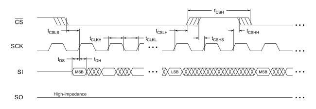
Figure 14-2. Serial Output Timing
