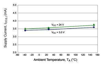
A1150/A1152/A1153/A1155/A1156/A1157/A1158 Average Supply Current (High) versus Temperature
