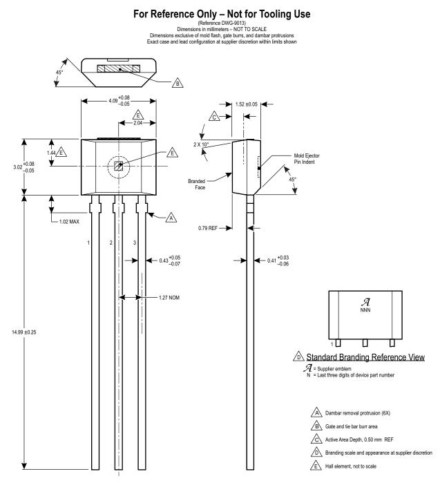
Figure 5: Package UA, 3-Pin SIP
