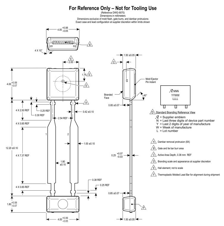
Figure 6: Package UB, 2-Pin SIP
