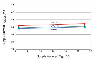
A1150/A1152/A1153/A1155/A1156/A1157/A1158 Average Supply Current (High) versus Supply Voltage
