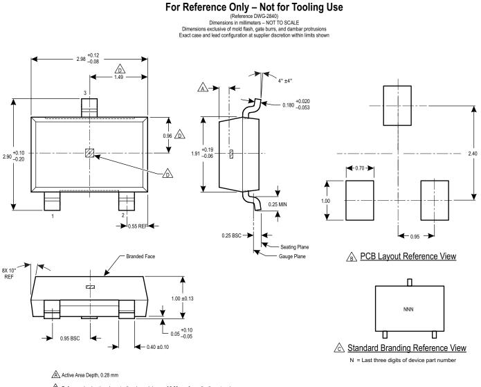
Reference land pattern layout; all pads a minimum of 0.20 mm from all adjacent pads; adjust as necessary to meet application process requirements and PCB layout tolerances
