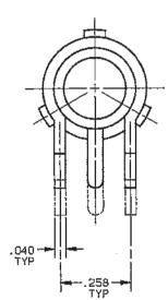
PRE-TINNED, .0015 MAXIMUM THICKNESS WITH SN63 OR EQUIV SOLDER, PER GG-S-571, TO WITHIN .060 MAXIMUM OF SHOULDER, AFTER PLATING
