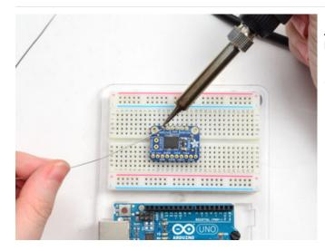
And Solder! Be sure to solder all pins for reliable electrical contact.
