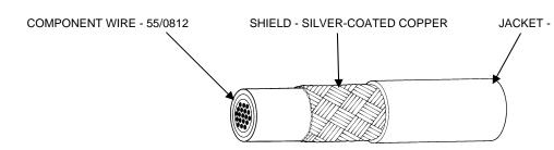
JACKET - LOW OUTGASSING, RADIATION-CROSSLINKED, MODIFIED ETFE
