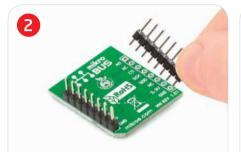
Turn the board upside down so that bottom side is facing you upwards. Place shorter parts of the header pins in both soldering pad locations.
