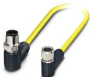
Sensor/actuator cable, 3-position, PVC, yellow, shielded, Plug angled M12 SPEEDCON, coding: A, on Socket angled M8, cable length: 1.5 m
