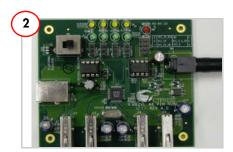
Plug the wall mounted power supply into an AC power receptacle providing power in the range 100 V to 240 V, 50 Hz or 60 Hz. Connect the power supply plug to the hub's 'DC Supply' jack.
