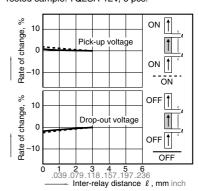
11. Pulse dialing test (35 mA 48 V DC wire spring relay load) Tested sample: TQ2SA-12V, 6 pcs. Circuit
