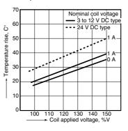
6. Ambient temperature characteristics Tested sample: TQ2-12V, 5 pcs.
