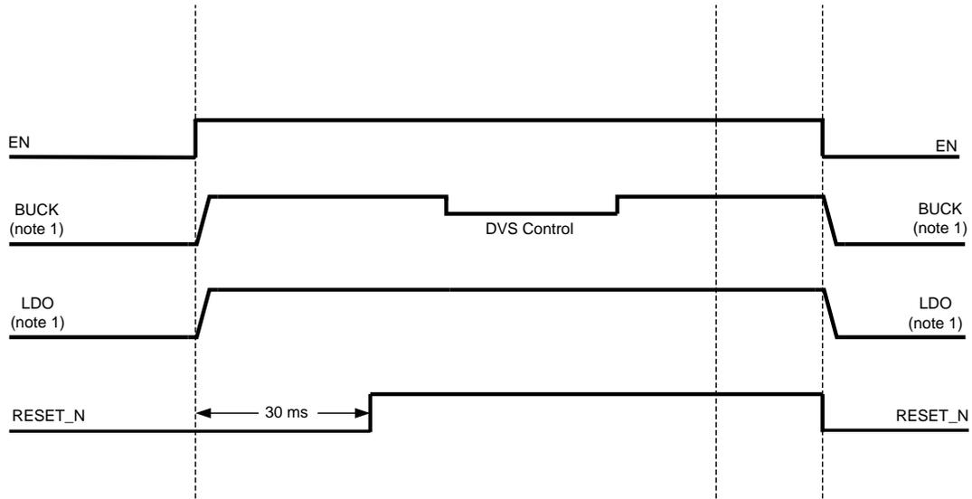
**Figure 3. Simplified startup Sequence if CONFIG=GND (SUB\_PMU)**
