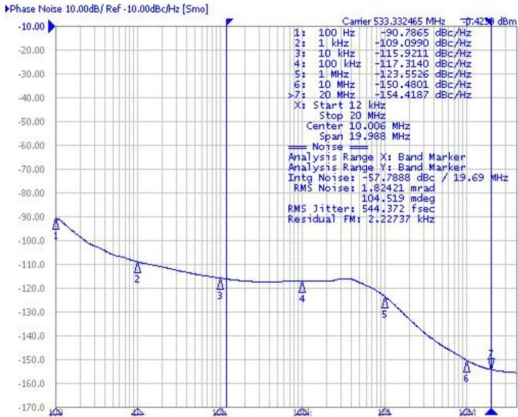
Figure 3. Typical Phase Noise Plot
