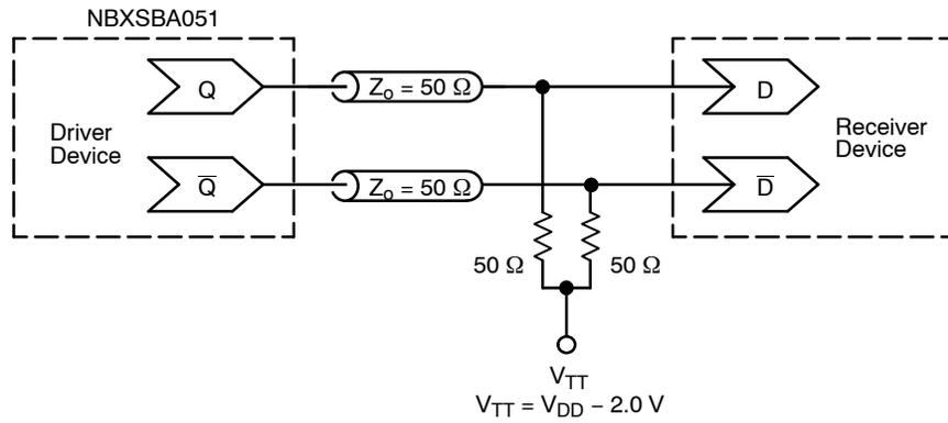
**Figure 4. Typical Termination for Output Driver and Device Evaluation**
