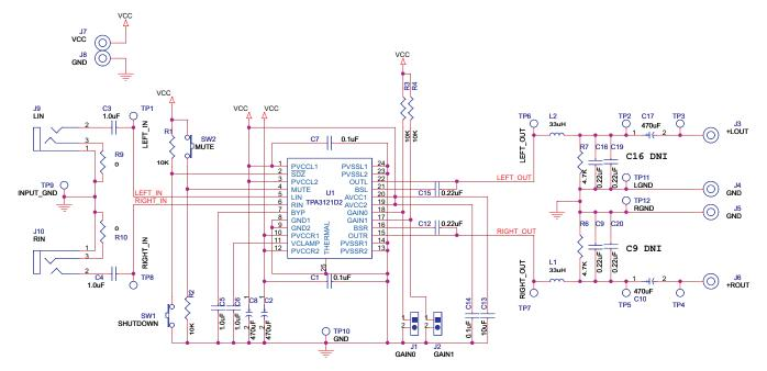
Figure 3. TPA3121D2 EVM Schematic
