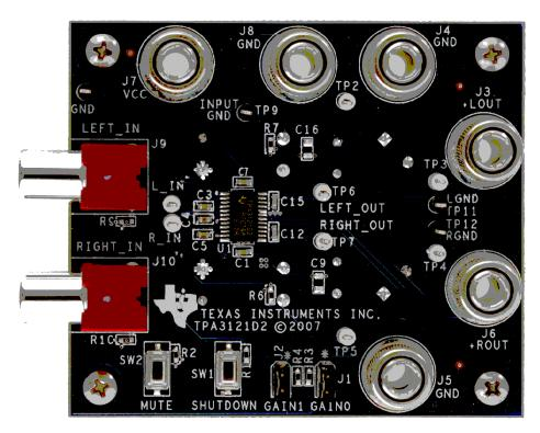
Figure 1. The TI TPA3121D2 Audio Power Amplifier EVM - Top View
