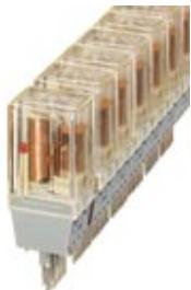
Relay connector, equipped with Hengstler miniature round relay, contacts (AgCdO+Au): small to large loads, 2 N/O contacts, input voltage 24 V DC, with light indicator, can be plugged on basic termination blocks
