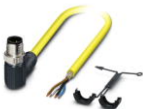
Sensor/actuator cable, 4-position, PVC, yellow, shielded, Plug angled M12 SPEEDCON, A-coded, on free cable end, cable length: 2 m
