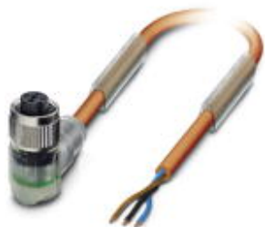
Sensor/actuator cable, 3-position, PUR halogen-free, irradiated, orange RAL 2003, free cable end, on Socket angled M12, A-coded, with 2 LEDs, cable length: 5 m, Customer-specific version
