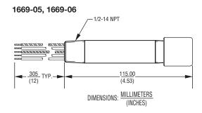
The 'single ended' protectors are useful for field devices with dual conduit ports; the field wiring connects to one port while the 1669 protector connects into the second - all connections are made within the instrument's wiring cavity. This installation simplifies the task of maintenance or of adding a protector into an existing loop.
