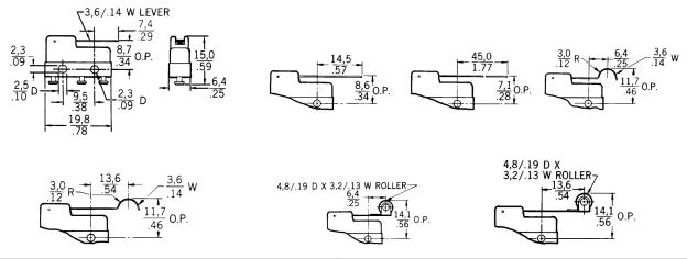
NOTE: The two mounting holes accept pins or screws of 2,21 mm (0.087 in) maximum diameter
