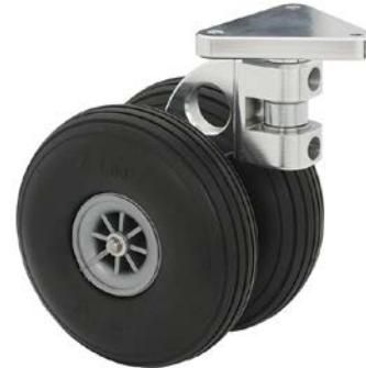
This kit contains a single, precision machined caster assembly (two are required if you're mounting them to our Arlo Robot Base Kit - #28960). High quality 6061 machined aluminum components are combined with smooth-rolling ball bearings and durable 3-inch pneumatic rubber tires. The dual independent tire design reduces vibration and drag, as well as increases load-carrying capacity.
