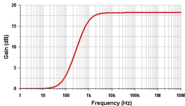
Note that the high-pass filter function is not a true high-pass filter. C2 in series with R23 creates a zero at about 10 Hz. As the frequency decreases from about 3 kHz to 10 Hz, the circuit changes from a gain stage into two unity gain buffers.
