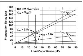
FIGURE 2-35: Propagation Delay vs. Load Capacitance.
