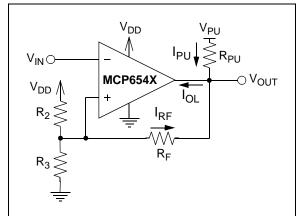
FIGURE 4-4: Inverting Circuit with Hysteresis.
