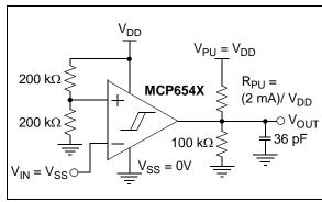
**FIGURE 1-3:** AC and DC Test Circuit for the Open-Drain Output Comparators.
