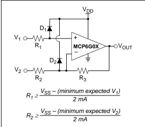
FIGURE 4-2: Protecting the Analog Inputs.
