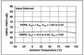
**FIGURE 2-13:** CMRR,PSRR vs. Ambient Temperature.
