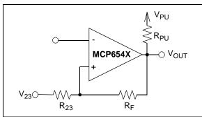
FIGURE 4-6: Thevenin Equivalent Circuit.
