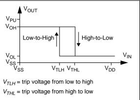
FIGURE 4-5: Hysteresis Diagram for the Inverting Circuit.
