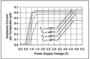
**FIGURE 2-17:** Quiescent Current vs. Power Supply Voltage.
