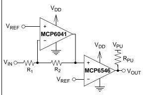
FIGURE 4-9: Precise Inverting Comparator.
