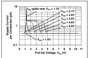
FIGURE 2-19: Supply Current vs. Pull-Up Voltage.
