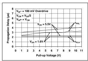
**FIGURE 2-33:** Propagation Delay vs. Pull-up Voltage.
