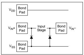
FIGURE 4-1: Simplified Analog Input ESD Structures.
