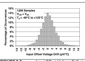
**FIGURE 2-2:** Input Offset Voltage Drift at  $V_{CM} = V_{SS}$ .
