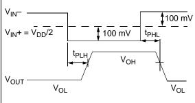
FIGURE 1-2: Propagation Delay Timing Diagram.
