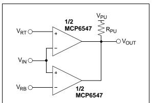
FIGURE 4-10: Windowed Comparator.
