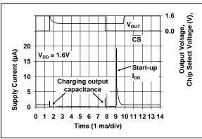
**FIGURE 2-38:** Supply Current (Charging Current) vs. Chip Select (CS) pulse at  $V_{DD} = 1.6V$  (MCP6548 only).
