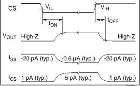
FIGURE 1-1: Timing Diagram for the CS pin on the MCP6548.
