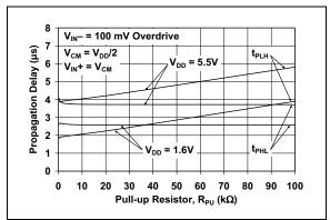
**FIGURE 2-32:** Propagation Delay vs. Pull-up Resistor.
