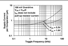
FIGURE 2-20: Supply Current vs. Toggle Frequency.
