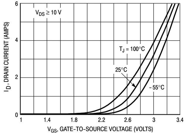
Figure 2. Transfer Characteristics
