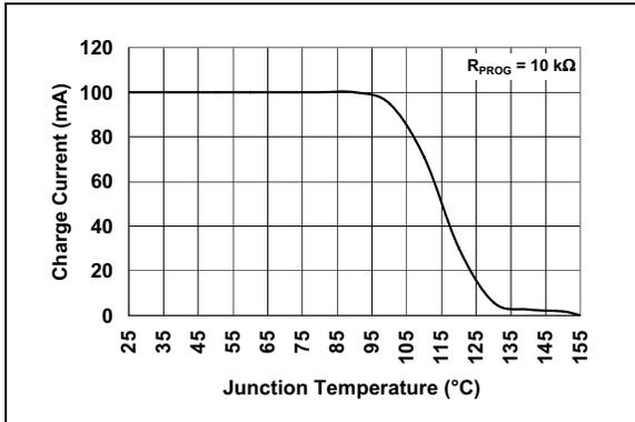
**FIGURE 2-7:** Charge Current ( $I_{OUT}$ ) vs. Junction Temperature ( $T_J$ ).
