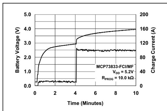
FIGURE 2-18: Charge Cycle Start - Preconditioning (180 mAh Li-Ion Battery).
