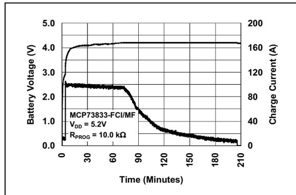
FIGURE 2-17: Complete Charge Cycle (180 mA Li-Ion Battery).
