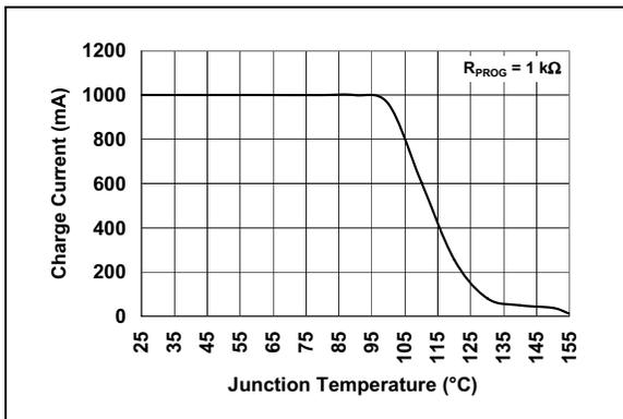
**FIGURE 2-8:** Charge Current ( $I_{OUT}$ ) vs. Junction Temperature ( $T_J$ ).
