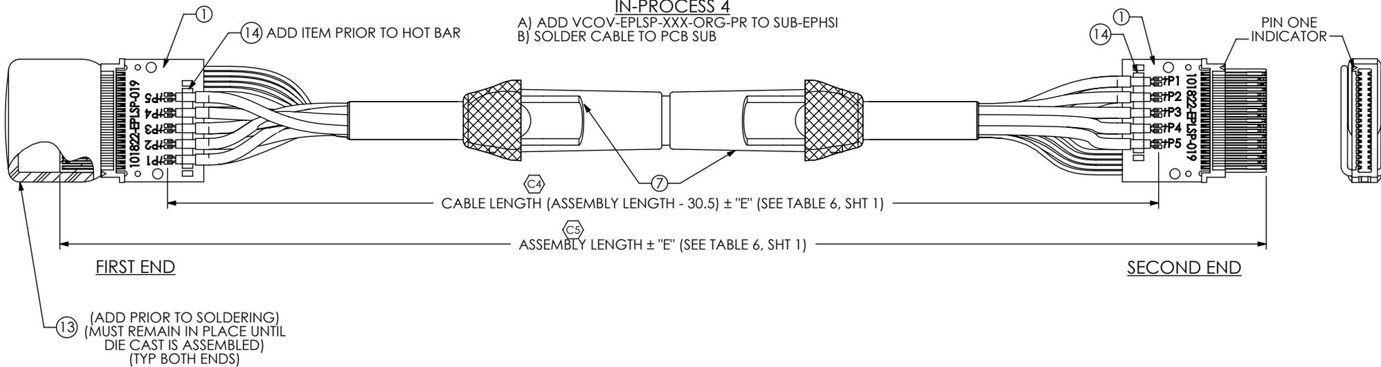
**NOTE: CABLE 2 FOR -031 POSITION WILL NEED PAIR 2 & 5 DISCRETE WIRES CUT BACK TO SHIELD.**
