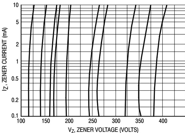
Figure 9.  $V_Z = 100$  thru 400 Volts
