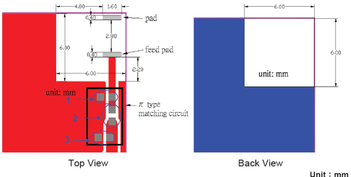
Matching circuit: (Center frequency is 5500MHz at 40x40mm ground plane)
