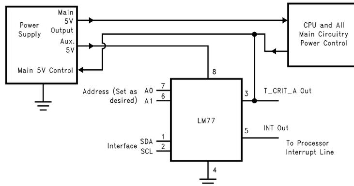
By powering the LM77 from auxiliary output of the power supply, a non-functioning overheated computer can be powered down to preserve as much of the system as possible.
