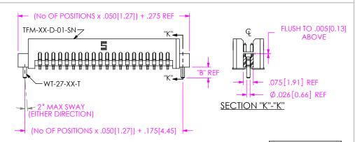
FIG 12 -SNX: SOLDER NAIL DIFFERENT AS SHOWN, OTHERWISE SAME AS FIG 1
