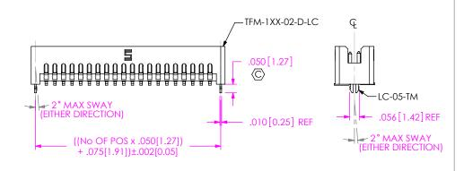
FIG 10 -LC OPTION DIFFERENT AS SHOWN, OTHERWISE SAME AS FIG 1 (NOT AVAILBLE ON -RA)
