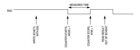
Figure 13-22. Bit Time Measurement with ACLK = 1, Scenario B
