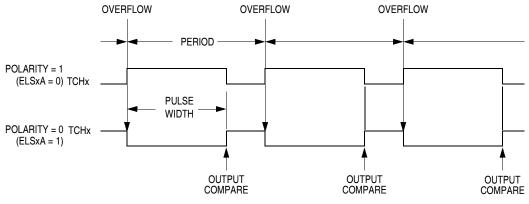
Figure 16-3. PWM Period and Pulse Width
