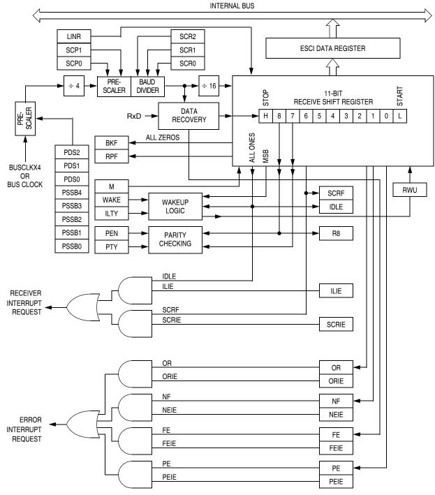
Figure 13-5. ESCI Receiver Block Diagram
