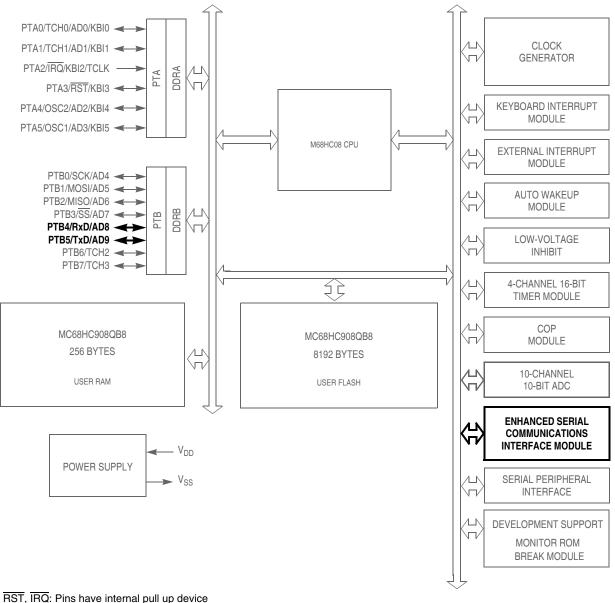
All port pins have programmable pull up device PTA[0:5]: Higher current sink and source capability
