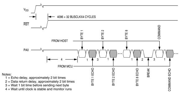
Figure 17-18. Monitor Mode Entry Timing
