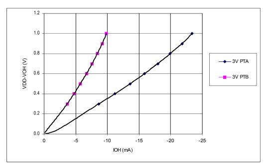
Figure 18-4. Typical 3-Volt Output High Voltage versus Output High Current (25°C)
