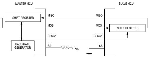
Figure 15-3. Full-Duplex Master-Slave Connections
