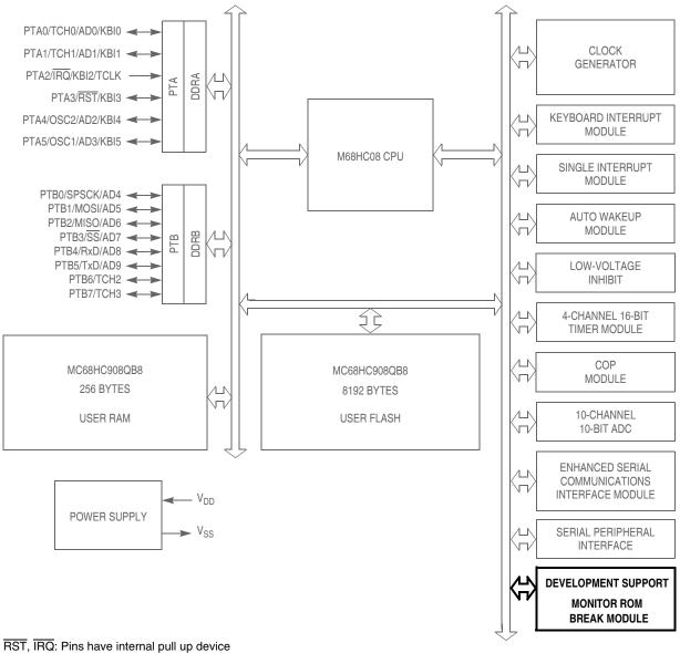
RST, IRQ: Pins have internal pull up device All port pins have programmable pull up device PTA[0:5]: Higher current sink and source capability
