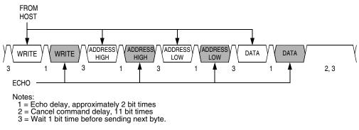
Figure 17-16. Write Transaction
