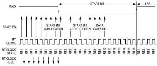
Figure 13-6. Receiver Data Sampling
