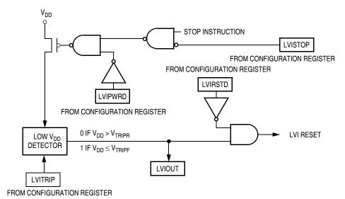
Figure 10-1. LVI Module Block Diagram
