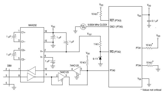
Figure 17-10. Monitor Mode Circuit (External Clock, with High Voltage)
