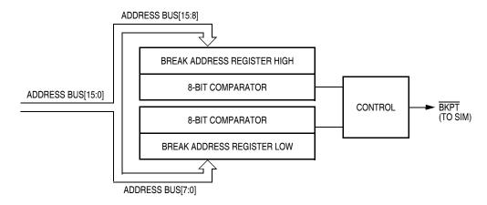
Figure 17-2. Break Module Block Diagram
