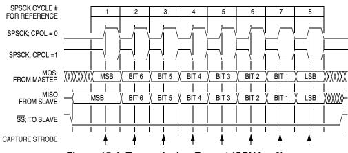
Figure 15-4. Transmission Format (CPHA = 0)
