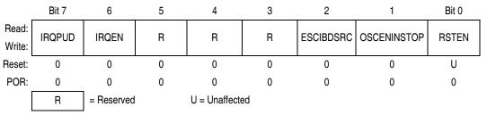
Figure 5-1. Configuration Register 2 (CONFIG2)
