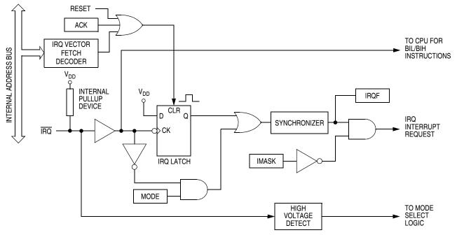
Figure 8-2. IRQ Module Block Diagram
