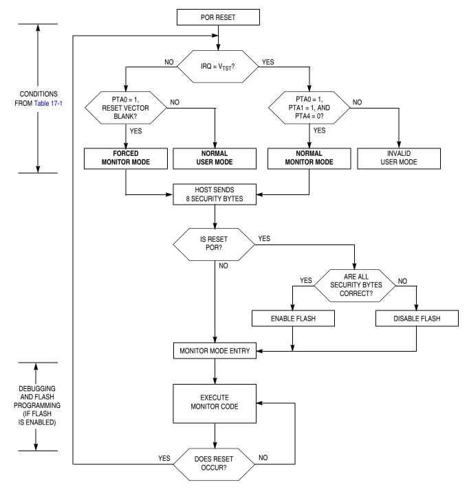
Figure 17-9. Simplified Monitor Mode Entry Flowchart
