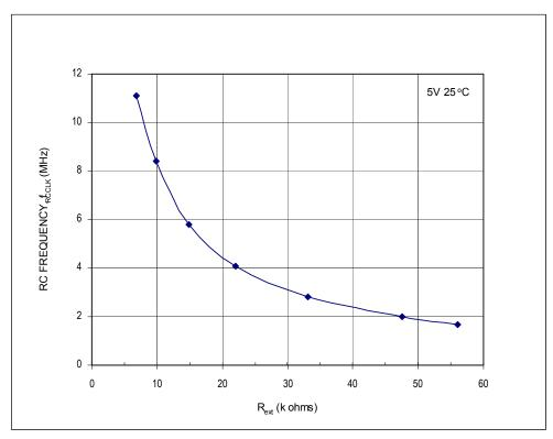
Figure 18-7. RC versus Frequency (5 Volts @ 25°C)
