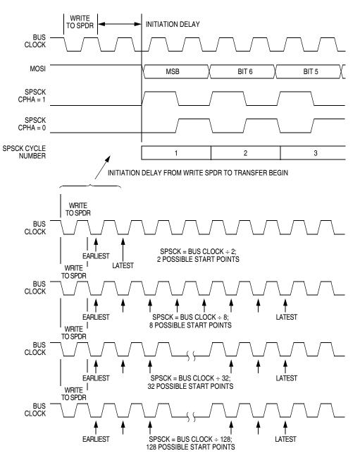
Figure 15-7. Transmission Start Delay (Master)
