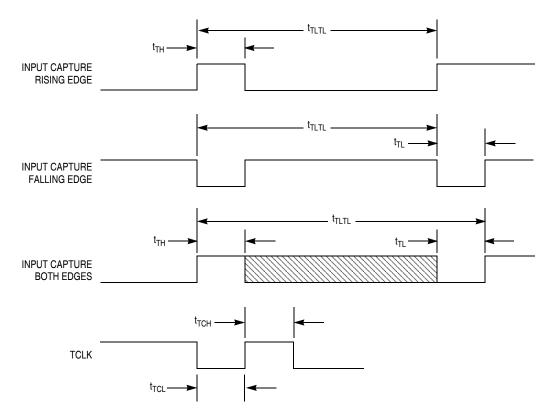
Figure 18-13. Timer Input Timing
