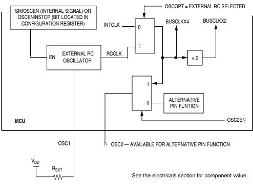
Figure 11-3. RC Oscillator External Connections
