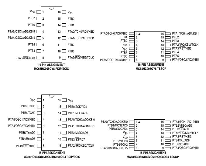
Figure 1-2. MCU Pin Assignments
