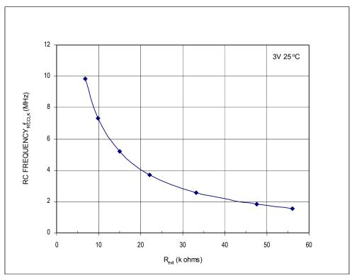
Figure 18-8. RC versus Frequency (3 Volts @ 25°C)
