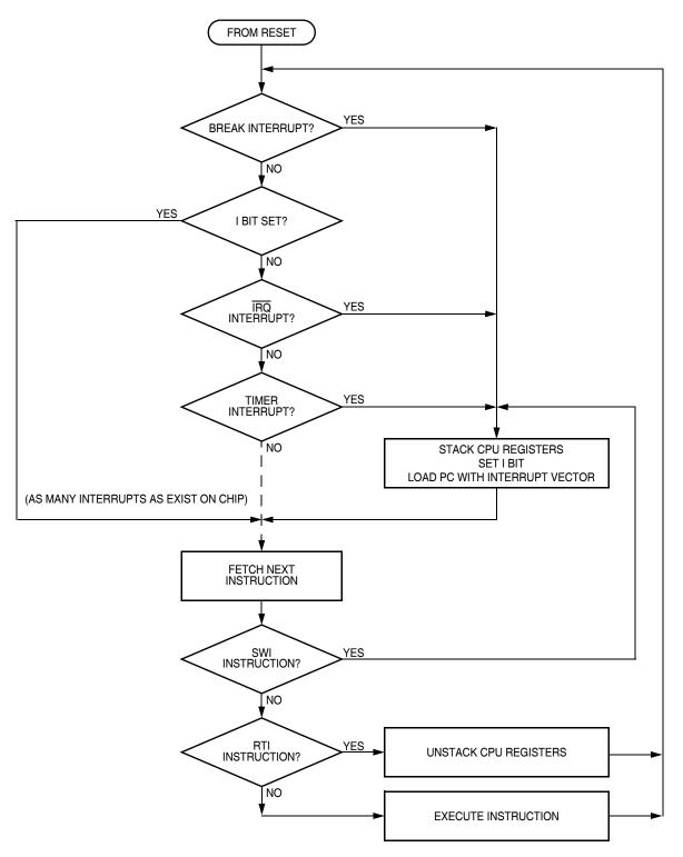
Figure 14-7. Interrupt Processing
