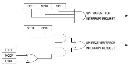
Figure 15-11. SPI Interrupt Request Generation
