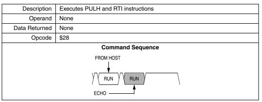
The MCU executes the SWI and PSHH instructions when it enters monitor mode. The RUN command tells the MCU to execute the PULH and RTI instructions. Before sending the RUN command, the host can modify the stacked CPU registers to prepare to run the host program. The READSP command returns the incremented stack pointer value, SP + 1. The high and low bytes of the program counter are at addresses SP + 5 and SP + 6.
