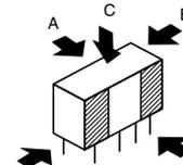
Please chuck the portion. Avoid chucking the center of the relay. In addition, excessive chucking pressure to the pinpoint of the relay should be avoided.
