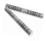
Tyco Electronics is a leading European supplier of high specification power resistors for specialist applications. The HVR range consists of high power, high voltage resistors capable of operating up to 50kV (continuous) and dissipating 50W in air or 100W oil. The thick film resistor element is designed to minimise inductance and capacitance giving optimum performance at MHz frequencies, and resistance to high voltage surges.
