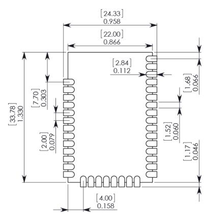
While the underside of the module is mostly coated with solder resist, we recommend that the copper layer directly below the module be left open to avoid unintended contacts. Copper or vias must not interfere with the three exposed RF test points on the bottom of the module (see below). Furthermore, these modules have a ground plane in the middle on the back side for shielding purposes, which can be affected by copper traces directly below the module.
