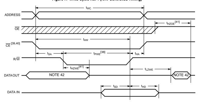
Figure 7. Write Cycle No. 1 (R/W Controlled Timing) [35, 36, 37, 38]
