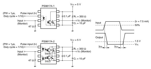
Remark CL includes probe and stray wiring capacitance.
