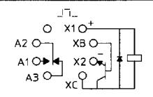
CONTACT RATING: LOW LEVEL TO 1A 28 VDC RESISTIVE 100,000 OPERATIONS
