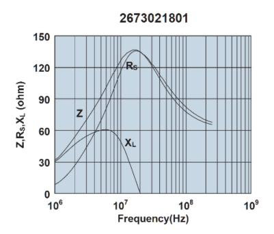
Impedance, reactance, and resistance vs. frequency.
