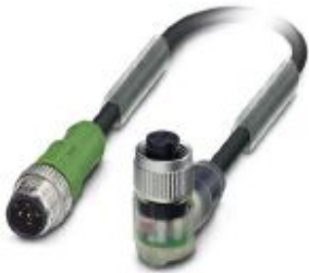
Sensor/actuator cable, 5-position, PUR halogen-free, black-gray RAL 7021, Plug straight M12, coding: A, on Socket angled M12, coding: A, with 3 LEDs, cable length: 0.6 m
