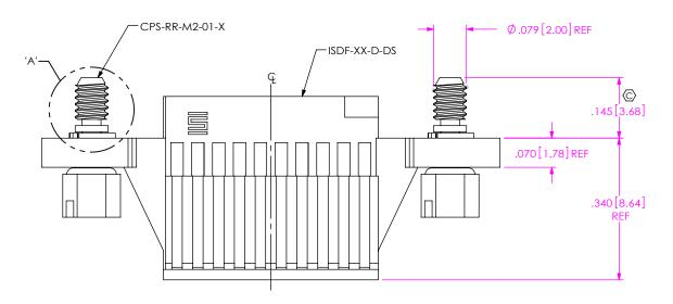
FIG 2 -S: DUAL SCREW DOWN OPTION ISDF-10-D-S SHOWN (DIFFERENT AS SHOWN, OTHERWISE SAME AS FIG 1)
