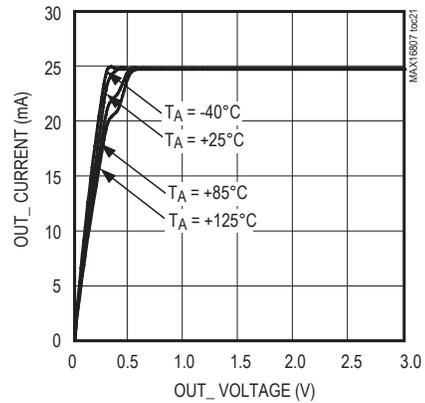
OUT\_ CURRENT vs. OUT\_ VOLTAGE
