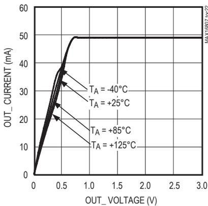
OUT\_ CURRENT vs. OUT\_ VOLTAGE
