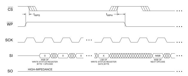
Figure 16-3. WP Timing for Write Status Register Byte 1 Command When SPRL = 1
