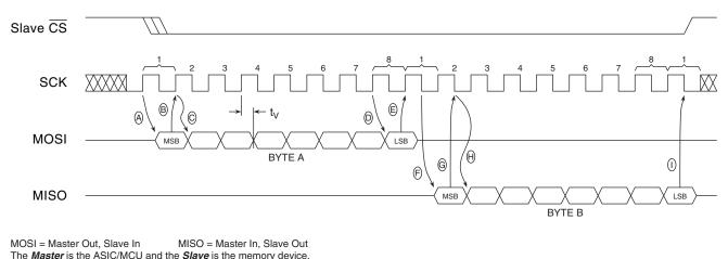
The *Master* always clocks data *out on the rising edge* of SCK and always clocks data in on the falling edge of SCK. The *Slave* always clocks data *out on the falling edge* of SCK and always clocks data in on the rising edge of SCK.
