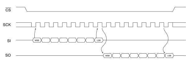
Figure 5-1. SPI Mode 0 and 3
