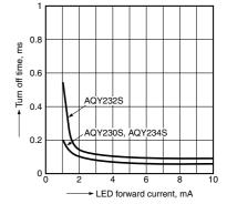
Sample: All types; Load voltage: Max. (DC); Continuous load current: Max. (DC)
