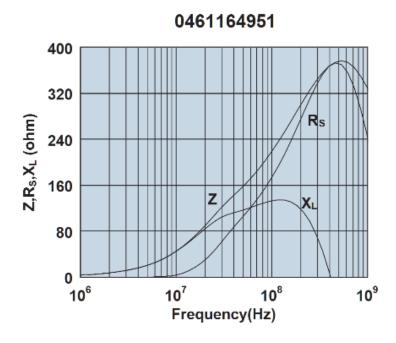
Impedance, reactance, and resistance vs. frequency.
