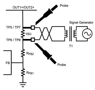
Figure 9. Loop Response Measurement Setup
