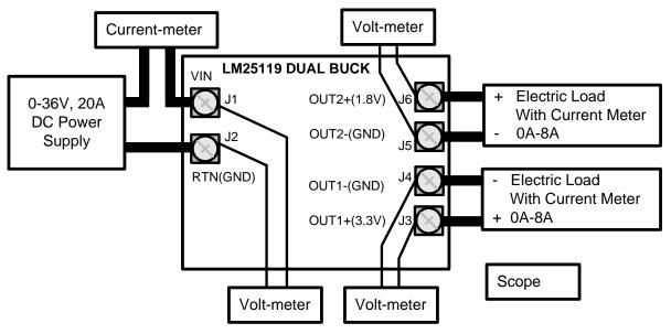
Figure 1. Typical Evaluation Setup
