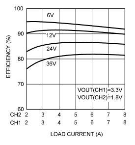
Figure 7. Typical Efficiency vs Load Current
