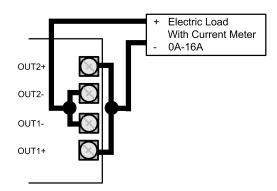
Figure 8. Load Connection for Single Output
