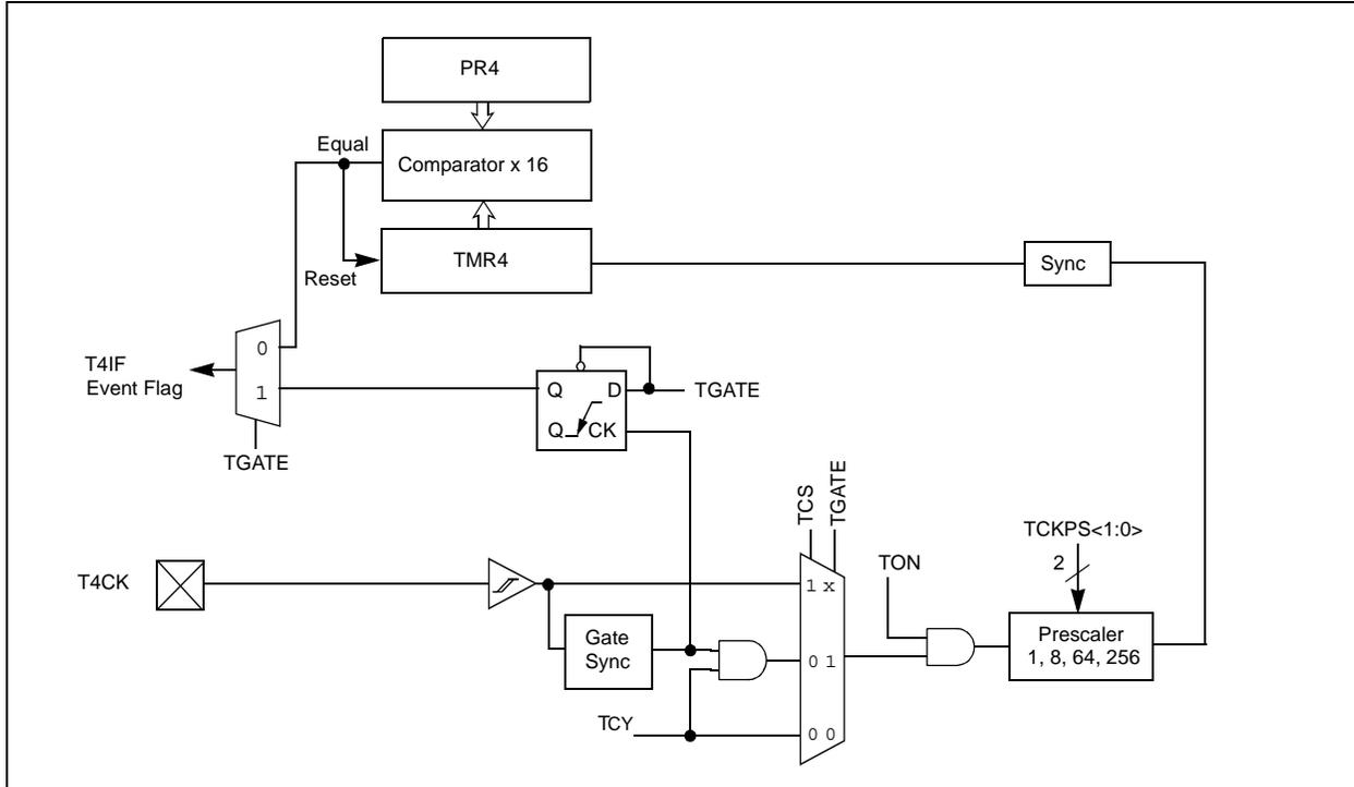
**FIGURE 11-3: 16-BIT TIMER5 BLOCK DIAGRAM (TYPE C TIMER)**
