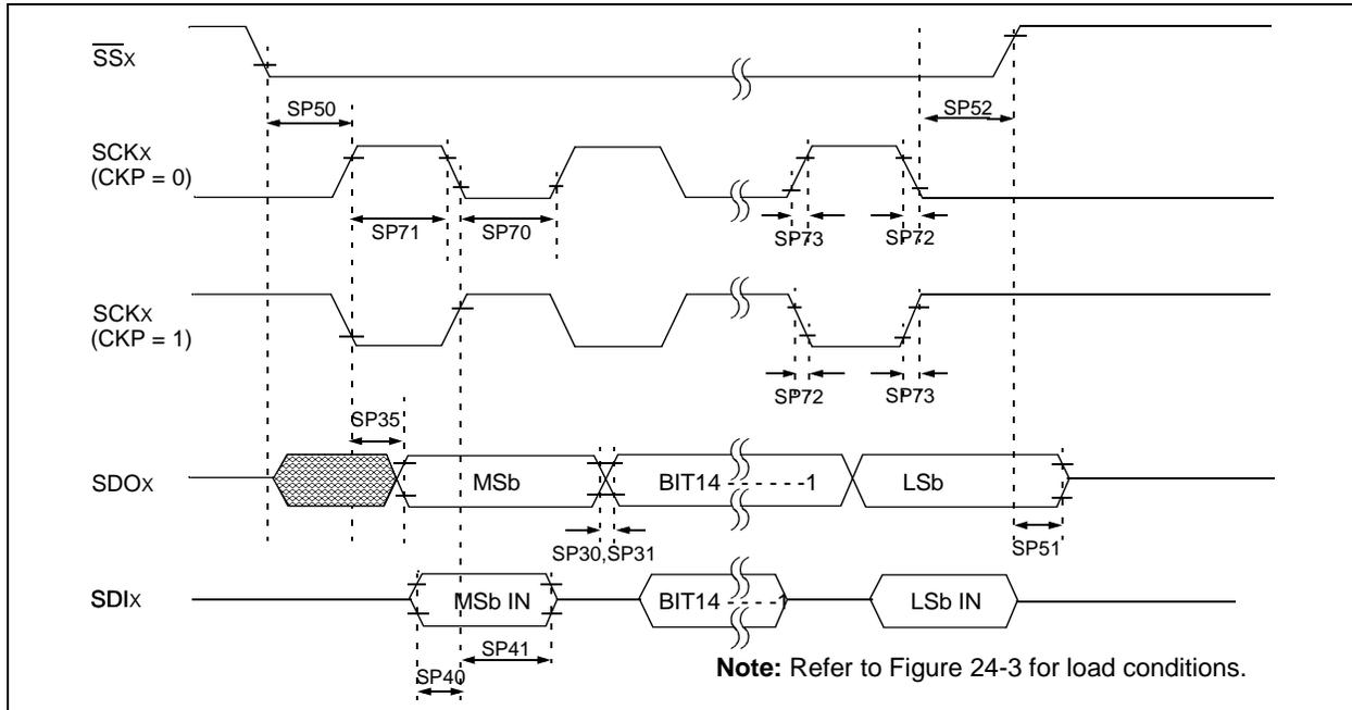
**TABLE 24-35: SPI MODULE SLAVE MODE (CKE = 0) TIMING REQUIREMENTS**
