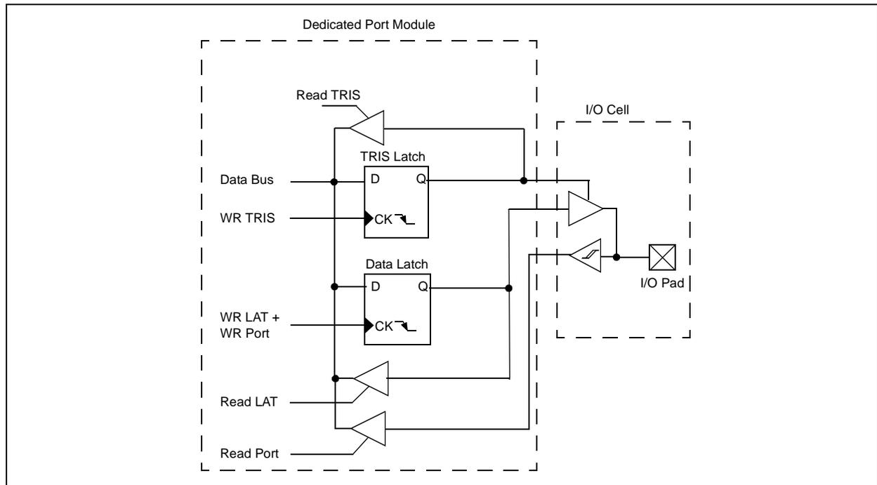
**FIGURE 8-2: BLOCK DIAGRAM OF A SHARED PORT STRUCTURE**
