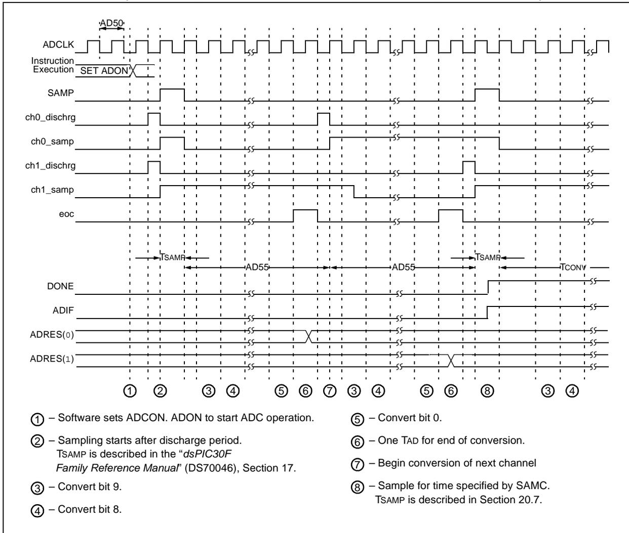
**TABLE 24-41: 10-BIT HIGH-SPEED ADC CONVERSION TIMING REQUIREMENTS**
