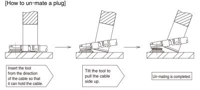
Never un-mate the plug by pulling the cable. It may cause a failure of the connector.
