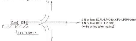
When the cable is routed in such a direction that lifts the cable, it is recommended that cushioning should be placed on the plug to prevent the connector from unmating (see the example below).
