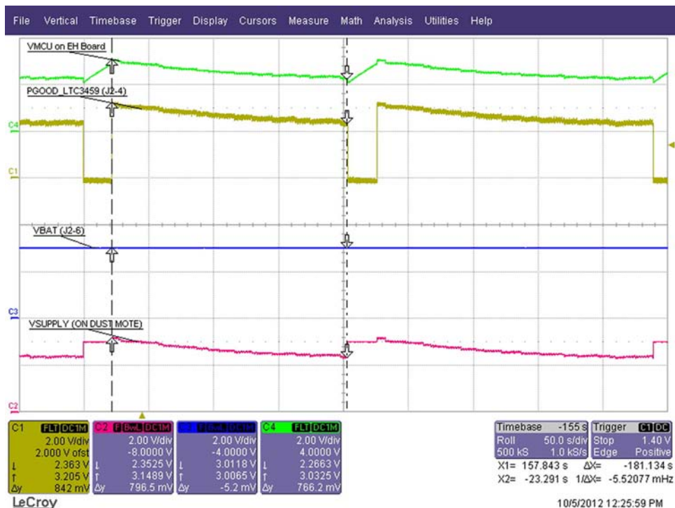
Figure 16. DC2042A LTC3459 Operation at 275 lux with Indy4100 Solar Panel
