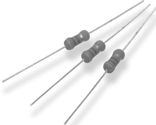
The resistive element comprises a metal oxide film deposited on a ceramic former. The element is protected by a flameproof coating which will withstand overload conditions without flame or mechanical damage. They are recommended for use in applications such as line protection etc...
