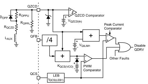
Figure 27. Overpower Compensation Circuit Schematic
