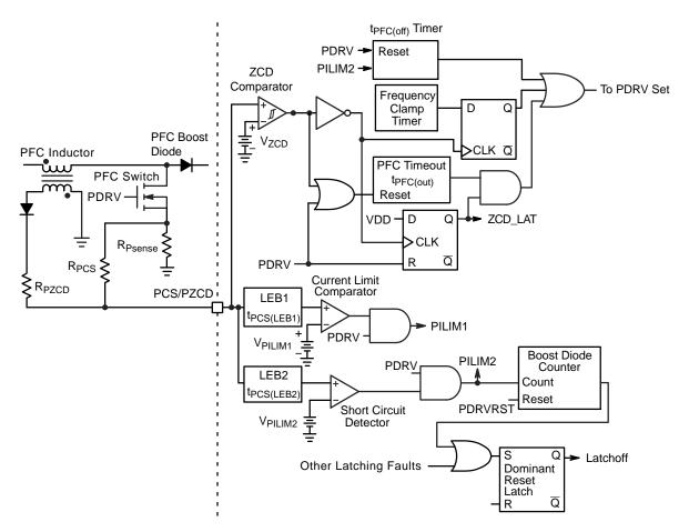
Figure 32. PFC Current Sense and ZCD Detectors Schematic
