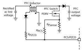
Figure 33. ZCD Winding Implementation
