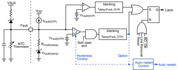
Figure 9. Fault Detection Schematic
