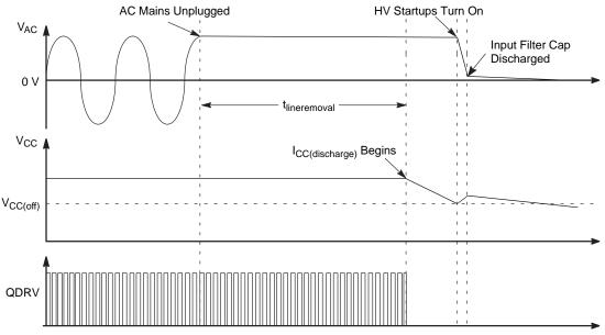
Figure 6. Input Filter Capacitor Discharge Waveforms
