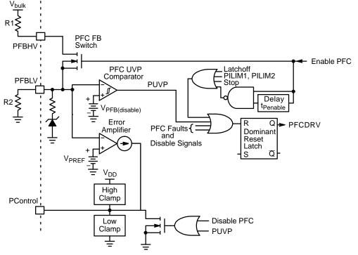
Figure 30. PFC Regulation Circuit Schematic
