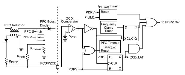
Figure 35. PFC Frequency Clamp Schematic
