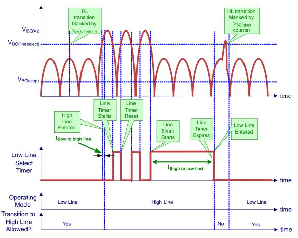
Figure 5. Line Detector Waveforms
