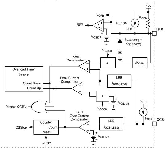
Figure 24. Current Sensing Circuitry Schematic
