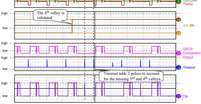
Figure 23. Timeout Operation with Missing 3<sup>rd</sup> and 4<sup>th</sup> Valleys
