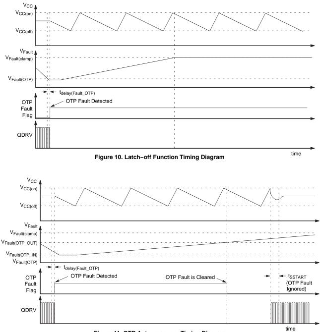
Figure 11. OTP Auto-recovery Timing Diagram
