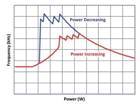
Figure 12. Valley Lockout Frequency vs. Output Power Relationship
