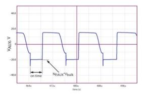
Figure 28. Auxiliary Winding Voltage Waveform
