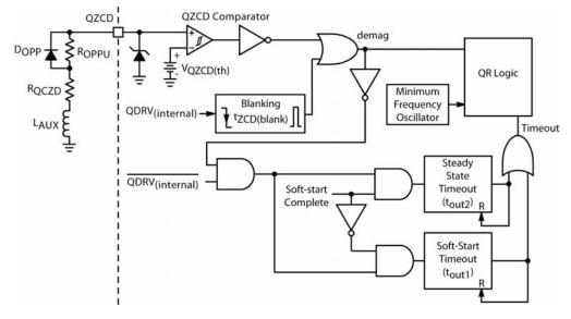
Figure 21. Timeout Period Generator Circuit Schematic
