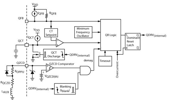
Figure 13. Valley Lockout Detection Circuitry Internal Schematic
