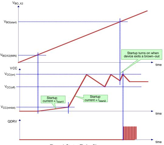
Figure 4. Startup Timing Diagram
