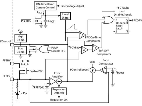
Figure 31. Boost and Soft–OVP Circuit Schematics
