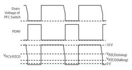
Figure 34. ZCD Winding Waveforms
