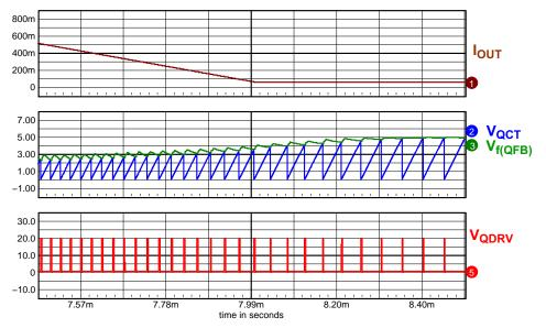
Figure 20. VCO Mode Operating Waveforms
